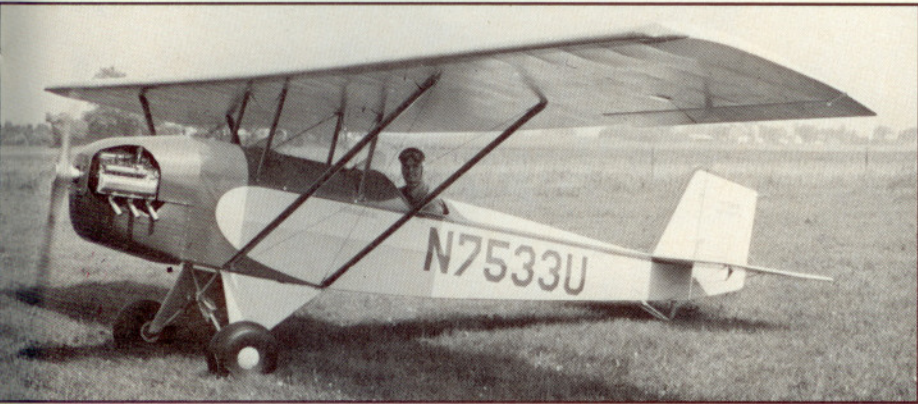
Pietenpol built this Air Camper in 1965. It has an air-cooled Chevrolet Corvair engine, Piper Cub landing gear and a lengthened rear fuselage. The front cockpit is covered for solo flight.
