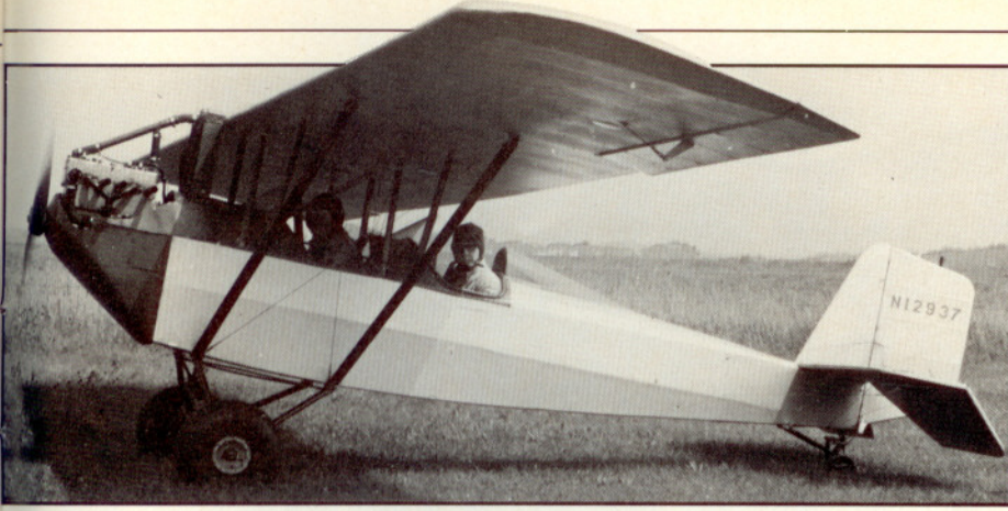
The revised 1933 Air Camper featured a new steel-tube landing gear and minor fuselage changes. This one was rebuilt in the 1960s with smaller main wheels and a steerable tailwheel.
